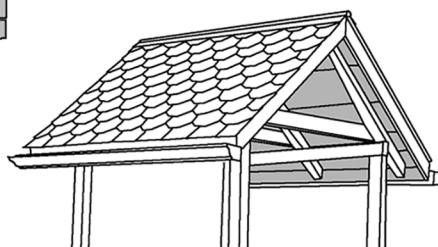
6. Install fascia boards, then the finished roofing. Recycled slate makes an excellent roofing material.
