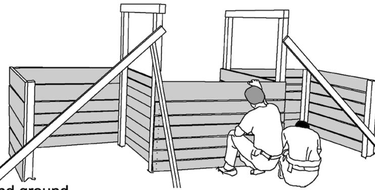
3. Screw 1" thick, rough sawn black locust (or other suitable) lumber to posts as shown. Leave small gap between boards and about 2" between bottom board and ground.
