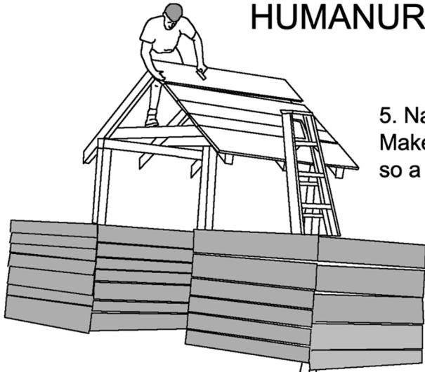
5. Nail sheathing boards to roof rafters. Make sure rafter tails have plumb cuts so a fascia board can be attached.
