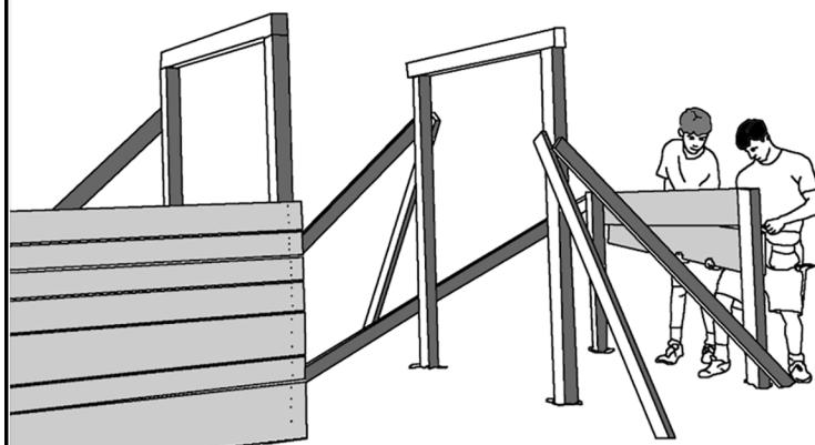
2. Plumb and brace posts. Nail 4x4 header across higher center posts.
