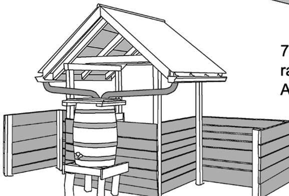
7. Install the rain spouting. Install a rain barrel adjacent to the Hacienda. A recycled oak wine barrel is an excellent rain water collector. Remember that you will have to drain the barrel during freezing weather.
