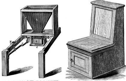
THE MECHANICAL PARTS OF THE COMMODE.
